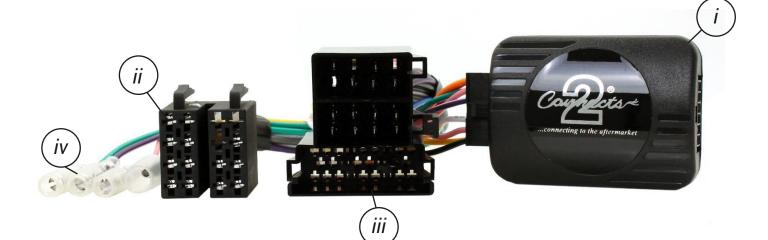
i. Interface Box ii. Male ISO Connector (16 Pin) iii. Mini ISO Connector iv. Flying Wires
