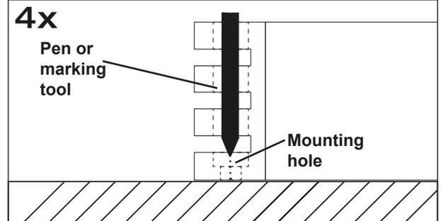
Keep the amplifier at the chosen mounting location in the vehicle. Then mark the four drill holes with an appropriate pen or marking tool through the designated mounting holes at the amplifier.
