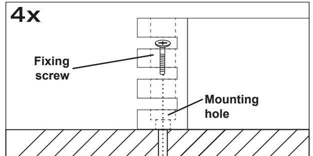
Then uphold the amplifier to the chosen position and fix the screws through the mounting holes into the drilled screw holes.
