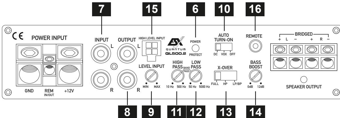
**6** If the **POWER/PROTECT** is blue, the amplifier is ready for operation. If the **POWER/PROTECT** is red, there is a malfunction. Refer in this case to the section **TROUBLE SHOOTING**.
