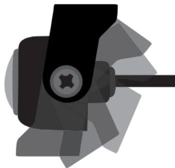
Fasten the camera in a suitable location either as a sub-assembly or surface-mounted camera. The bracket can be adjusted in several positions with 2 small screws.
