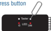
1. Press the programming button on the main unit and keep it pressed until the LED starts to flash rapidly. Release the button.
