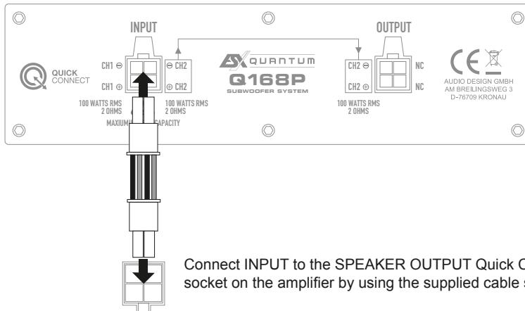
**Connection of two Q168P to a compatible amplifier with Quick Connect such as XE6440 DSP.**
