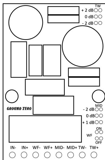
Tweeter level adjustment: The tweeter level can be set by positioning the jumper to the required level position
