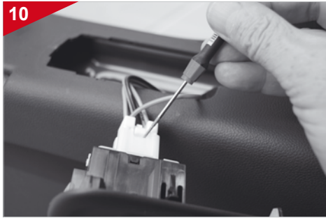
10 Remove the electric window connector and set it aside.
