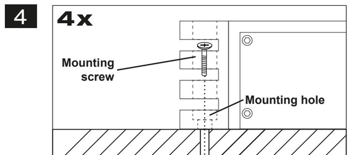
Then uphold the processor to the chosen position and fix the screws through the mounting holes into the drilled screwholes.
