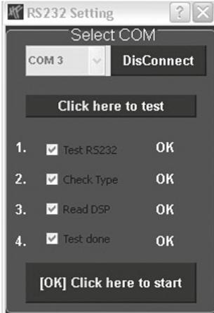
If the test was performed successfully 4 checkmarks in the check boxes appear. Then press **[OK]** [Click here to start](#) to continue.
