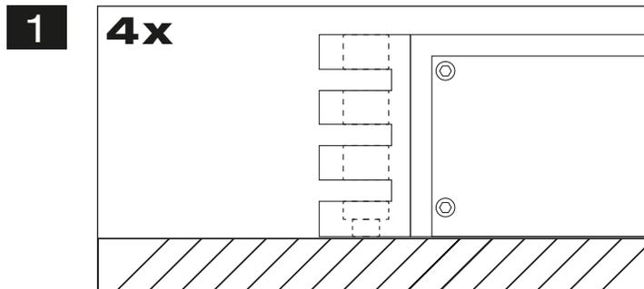
At first you need to find a suitable installation location for the processor. Ensure that enough space for the installation of the cables remains and that they will not be bended and have sufficient pull relief.
