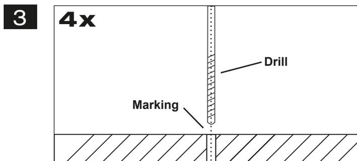
Lay the processor aside and then drill the holes for the mounting screws at the marked locations.
