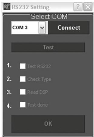
Enable the connection with the DSP in the **RS232 Setting**. The COM interface should be automatically detected and selected, it varies from system to system. Click then **Connect**. The program starts then automatically the connection.
