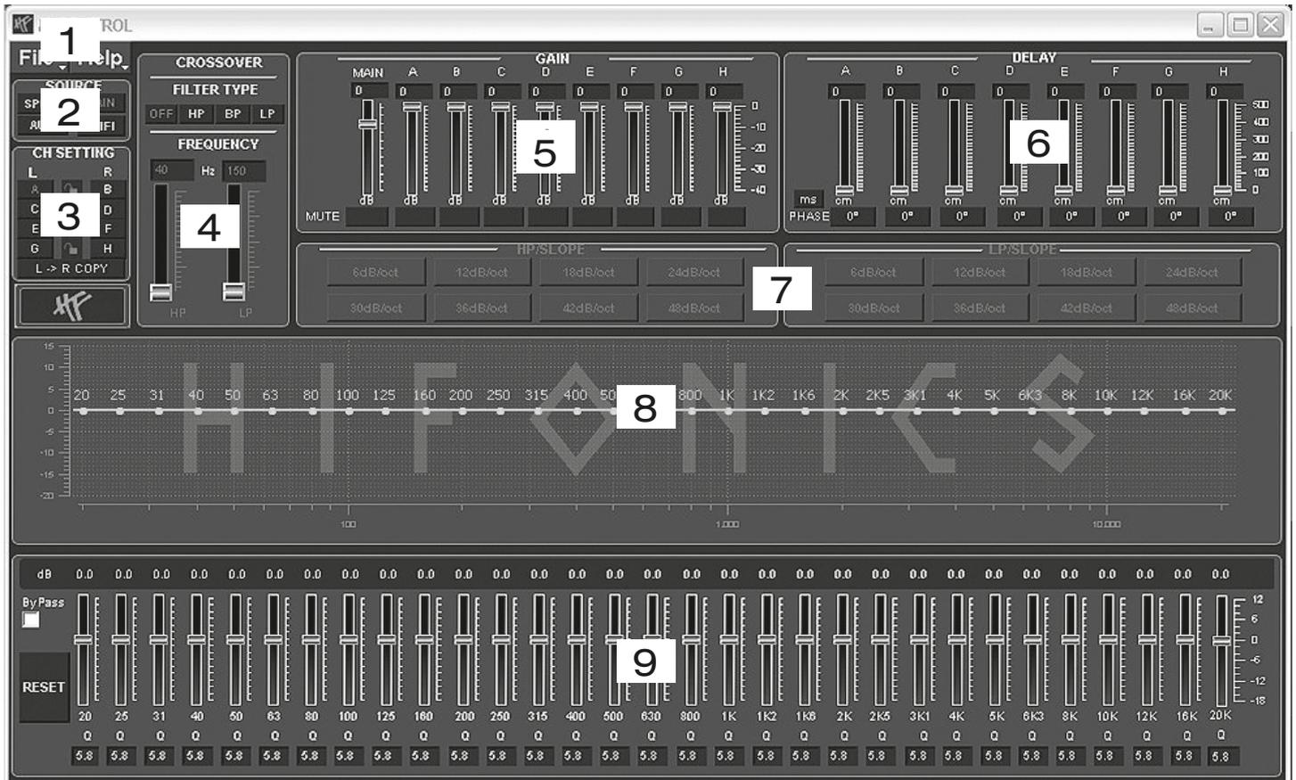
Here you are able to adjust many settings to customize your sound system, which are immediately audible in real time via the DSP processor. Once you are done with the configuration of a setting, it can be transferred to a storage space on the DSP processor. You can store up to 10 different settings and select them with the remote control at any time during operation.
