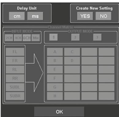
The configuration screen will appear next. Here you can determine how many RCA audio inputs you want to assign to the DSP processor and how these signals should be routed to speaker outputs.
