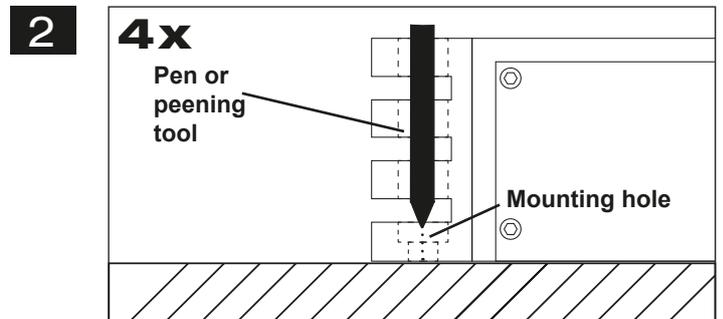
Keep the processor at the chosen mounting location in the vehicle. Then mark the four drill holes with an appropriate pen or peening tool through the designated mounting holes at the processor.
