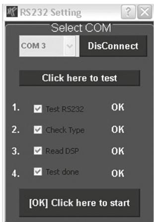
Click on **Click here to test** to check the connection with the DSP device.
