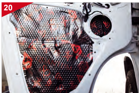
OPTIONAL: Then tape over the entire area that was previously covered with the white foam, which you can also use as a cutting template.
