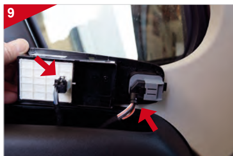
Carefully pull out the two plugs and then put the control panel aside.
