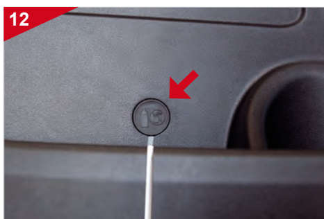
Remove the small round cover to the left of the cup holder and then remove the screw underneath.
