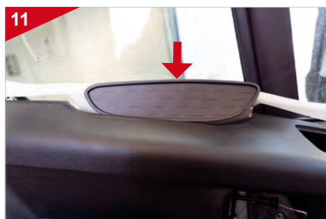
Lever out the rubber insert above the door handle, set it aside and remove the screw underneath.
