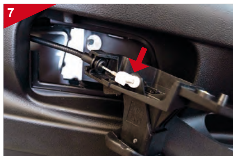
Pull the door handle and cable pull out of the opening. Detach the door handle from the cable and put the door handle aside.
