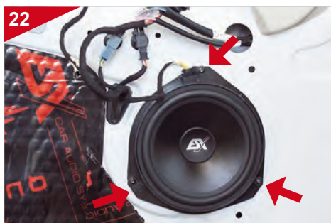
Insert the ESX speaker, fasten it with the three original screws and plug in the connector at the top.
