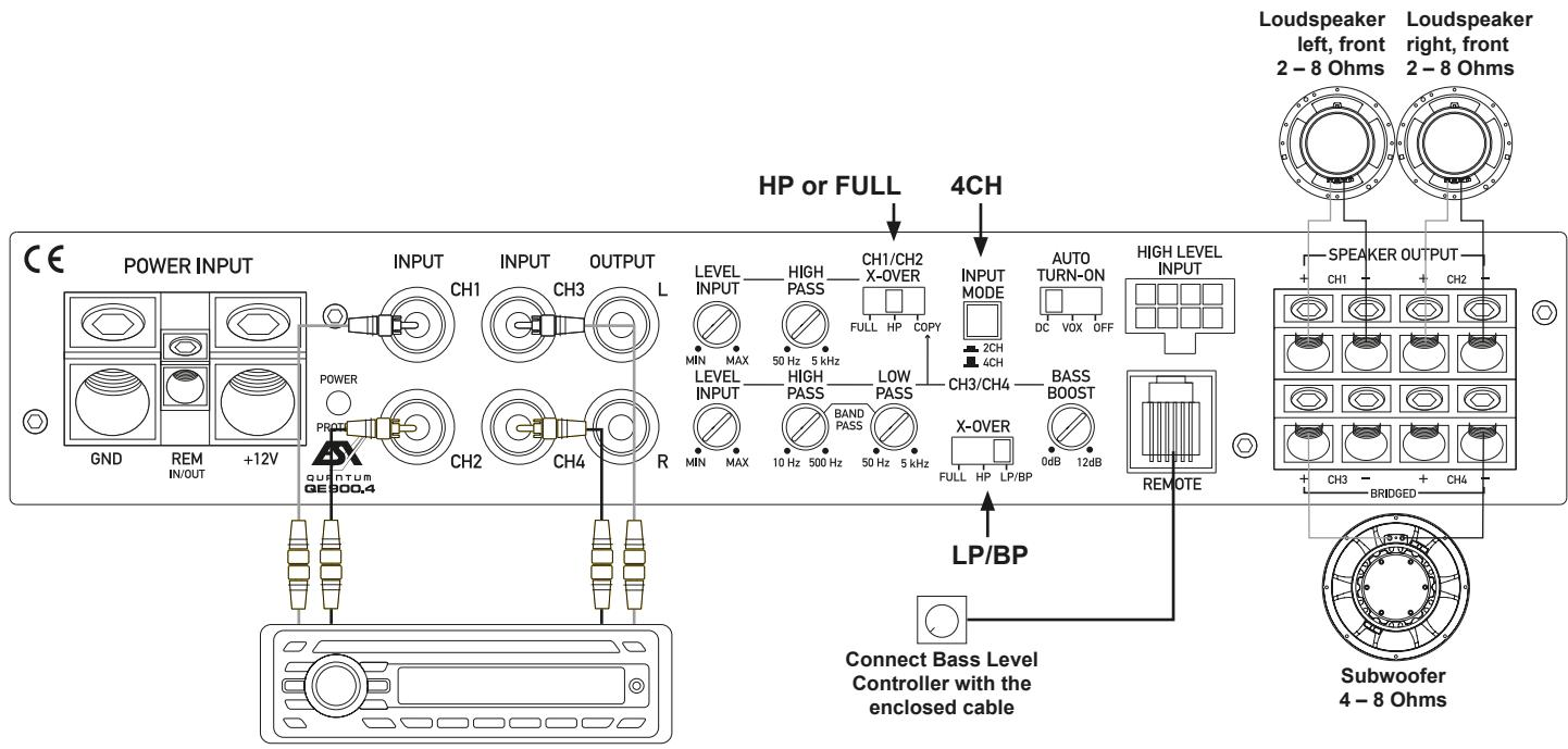
Connect stereo RCA outputs (FL/FR & RL/RR or SUB OUT) of the head unit with INPUT CH1 / CH2 and CH3 / CH4 of the amplifier
