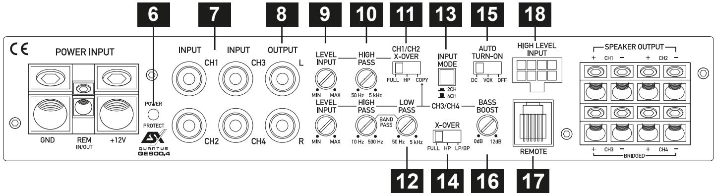
**6** If the **POWER/PROTECT** is blue, the amplifier is ready for operation. If the **POWER/PROTECT** is red, there is a malfunction. Refer in this case to the section **TROUBLE SHOOTING**.
