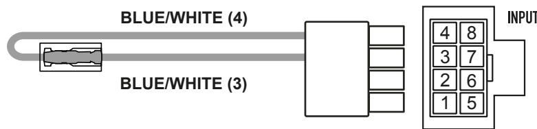
CONNECT THE BLUE/WHITE CABLES TO ACTIVATE THE AUTO TURN-ON FUNCTION.
