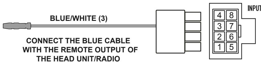
CONNECT THE BLUE CABLE WITH THE REMOTE OUTPUT OF THE HEAD UNIT/RADIO
