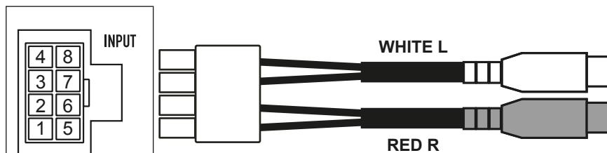
CONNECT THE RCA INPUTS WITH THE APPROPRIATE PRE-AMPLIFIER OUTPUTS OF THE HEAD UNIT/RADIO
