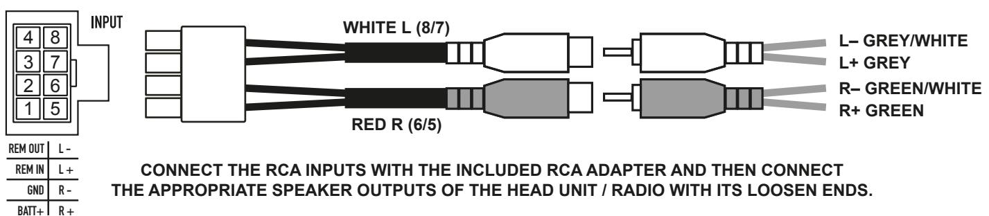
CONNECT THE RCA INPUTS WITH THE INCLUDED RCA ADAPTER AND THEN CONNECT THE APPROPRIATE SPEAKER OUTPUTS OF THE HEAD UNIT / RADIO WITH ITS LOSEN ENDS.
